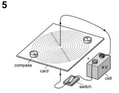
**6** The magnetic field produced by the current is very weak and it is even weaker the further you are from the wire. Therefore, a compass towards the edge of the card will be affected by the Earth's magnetic field as much as the wire's.
