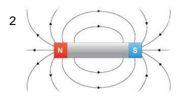
3 A permanent magnet produces its own magnetic field; an induced magnet becomes magnetic when placed in a magnetic field.
