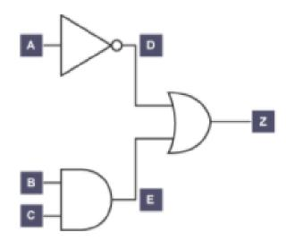
Altogether there are three inputs and eight possible outcomes. To solve the <u>truth table</u> below, first find D, then E and finally Z. Complete a whole columnn before moving on to the next column. D depends only on A, E depends on B and C, and Z depends on E or D.
