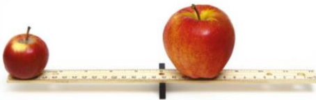
▲ These apples are in equilibrium because the clockwise moment equals the anticlockwise moment.
