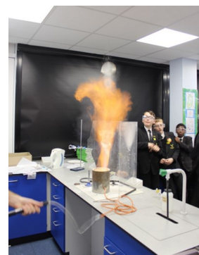
Figure 3 - Mr Wood demonstrating the explosive properties of powders - in this icing sugar
